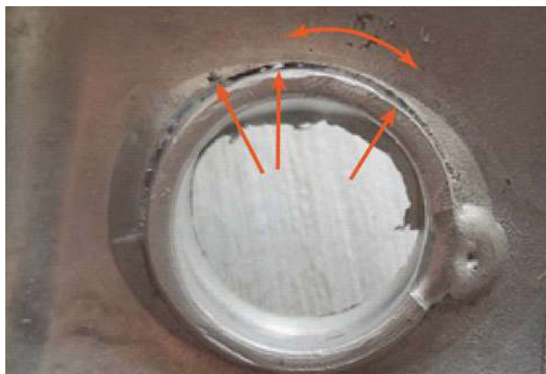
Fig. 6: BAD Welding – the weld seam is interrupted. The black coating from the outer shell might be visible.
